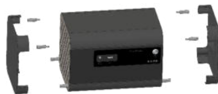
Fig. 24: Remove four distance bolts
