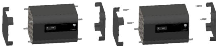
Fig. 24: Remove four distance bolts
